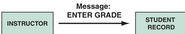
FIGURE 6-5 In a school information system, an INSTRUCTOR object sends an ENTER GRADE message to an instance of the STUDENT RECORD class.
